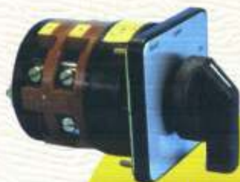
PANEL MOUNTING 3-POLE OFF-ON SWITCH FITTED WITH 88 x 88MM EXECUTION & TOGGLE KNOB MOUNTING THRO' 4 M6 SCREWS AT 68 CRS.
