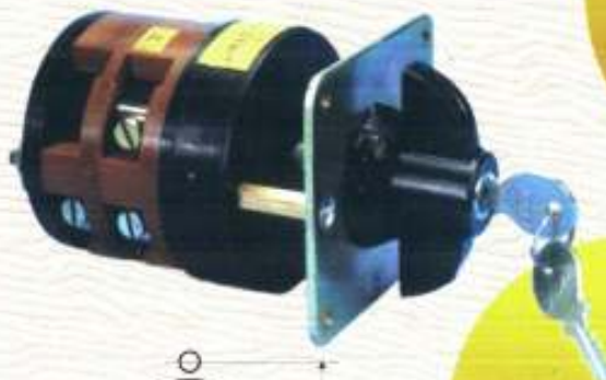
FITTED WITH WING TYPE KNOB LOCK ASSEMBLY KEY REMOVABLE IN ANY OF THE POSITIONS SWITCH MOUNTING THRO' 4 SCREWS OF M6 AT 68 CRS
